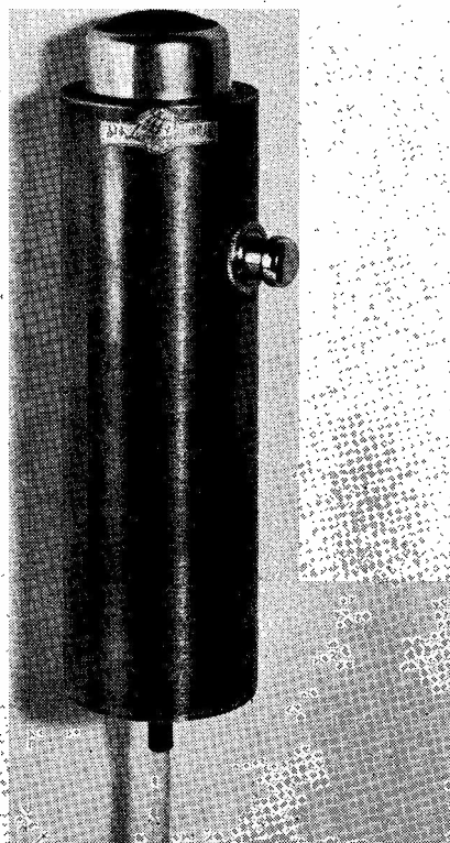
This is the Lustraphone D59/RT miniature microphone/transmitter, designed to work into the Lustraphone short-range communication system. It is an exceedingly interesting piece of apparatus, fully transistorised with the battery in the housing; all you do is to hold it, and speak; it has an automatic voice-operated gain control. The D59/RT is designed to work on the 175 mc band reserved for commercial services, and conforms to the G.P.O. specification for such apparatus.
